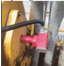
Gambar 5. Bracket sensor terpasang
